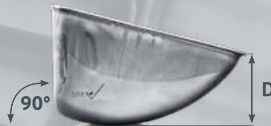
Bucket high front The bucket is placed vertically, and measured from the front and down
