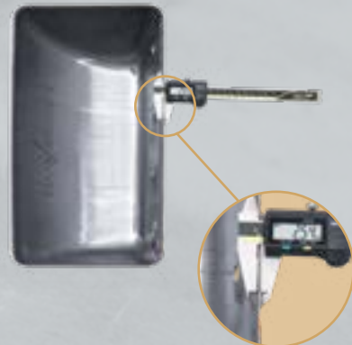
The thickness is measured with a caliper
